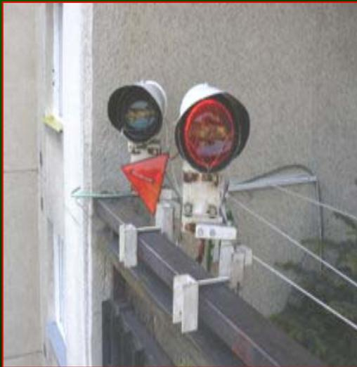
Ronja device installed on a balcony. The transmitter pipe (right) emits red light. The retroreflector triangle (left) is used for an initial aiming. The white steel holder allows precise adjustment of direction.
